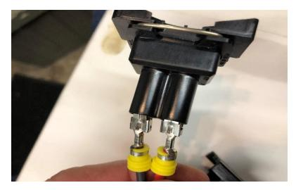
The ramps MUST be bent back into place before we reassemble the connectors into the housings.
