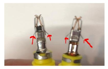
After all the ramps are in position align the wiring so that it lines up with the housing (as shown below) and insert each wire into the respective housing until you hear a click signifying the connector is in place.
