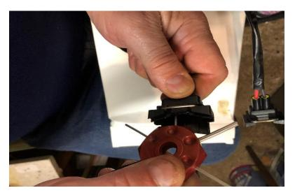
The wires fit snug in the connectors even when the ramps are compressed. It may require some finesse/wiggling to remove the pins from the housing. Make note of the wire colors/positions prior to disassembly.
