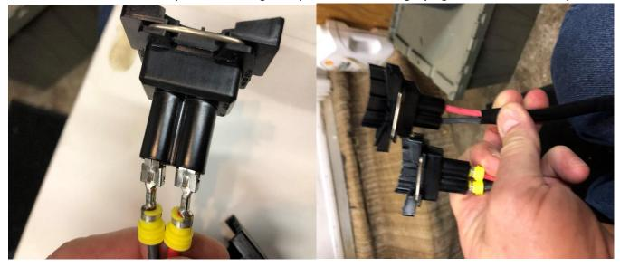
Once the pins are in place make sure the yellow moisture barriers are fully inserted.
