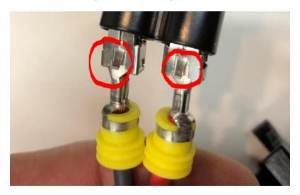
You may have to insert the tool several times before the ramps are successfully compressed far enough to allow the wires to pull out the back. Make note of the wire colors/positions prior to disassembly.
