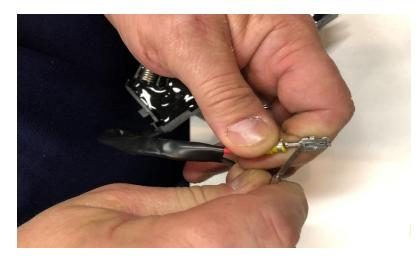
Ramps are shown bent out ready (below) for reassembly into the connector. We want about a 30-45 degree angle on the ramps to engage the locks in the housing when installed. Be careful not to bend these too far.
