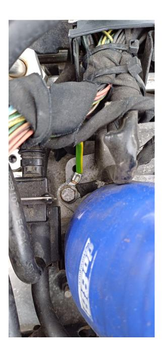
Add these 2 spacers on the original thread end of the throttle body bracket: see these 2 pictures below: (note: its demonstrated on top of the bracket but the spacers need to go below the bracket!):
