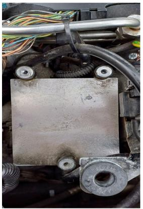
Place the ECU back on top of the 4 vibration dampers, secure the ecu with the delivered 18MM M6 bolts. Add the new ground cable to the top right corner of the ECU. Let the new ground cable go from top right corner bolt of the ECU to the top left corner bolt of the throttle body. Remove the Throttle body top left bolt (10 MM required), undo this bolt and connect the original ground cable and the new ground cable to this bolt. See picture below for reference:
