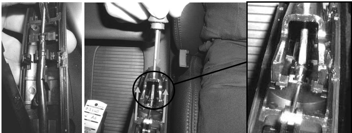
8. Hold the new lower shell to the metal frame of the hand brake lever. Starting from the rear, join the upper shell to the lower shell pressing firmly until all five clips are catching.
