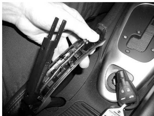
7. While mounting the new lower shell, hold the handbrake cable in place using a screw driver.
