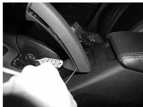
6. Remove the original lower shell, the release button and the spring. Take the new lower shell and install the handbrake cable into it. Install the cable and the spring into the release button.
