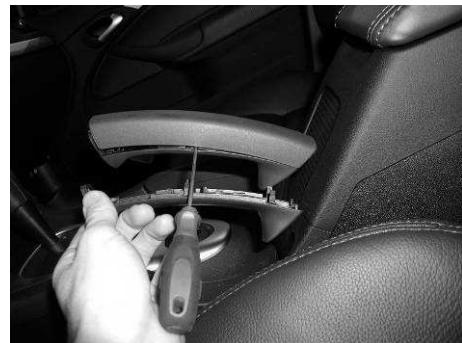
5. Release the rear clips and remove the original upper shell.
