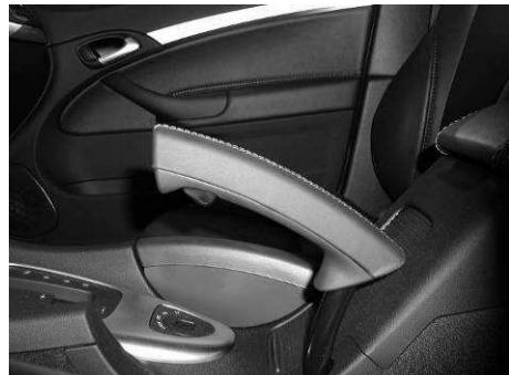
9. In some vehicles the handbrake lever might not align fully with the centre console when released. To adjust the alignment, pull the lever up and press it slightly to the correct side. Then release the lever and check the alignment. Repeat this procedure until the released lever is perfectly aligned with the centre console.
