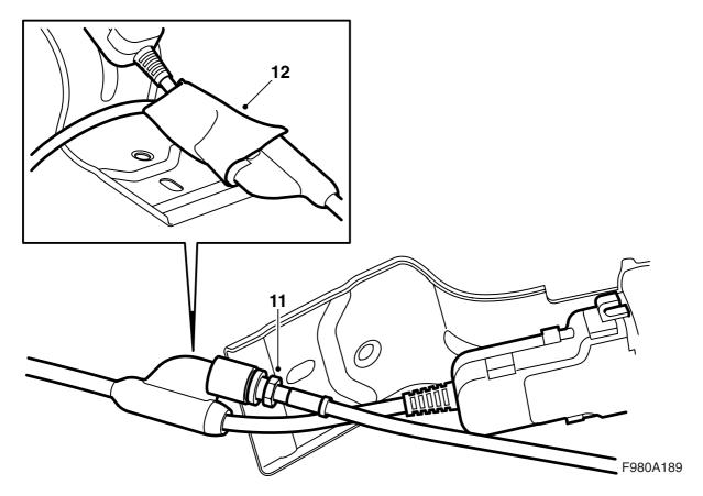
11 Run the antenna cable behind the dashboard support and connect it to the telephone holder cable antenna connection. Tighten the nut.
