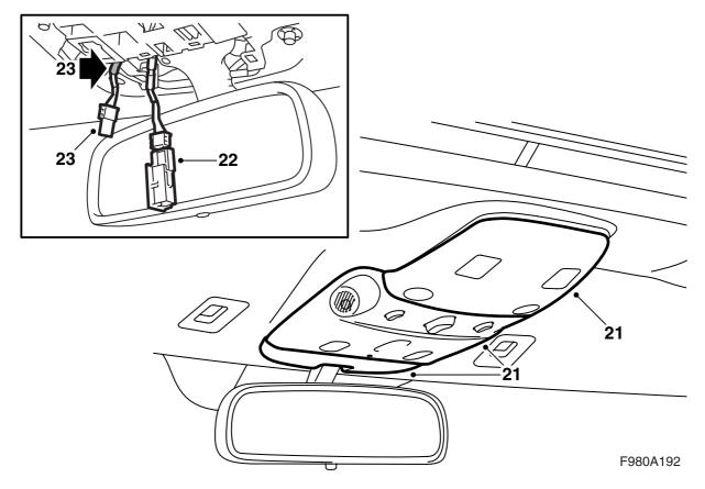
21 Remove the rear, centre and front sections of the roof lighting cover. Tool 82 93 474 is recommended.
