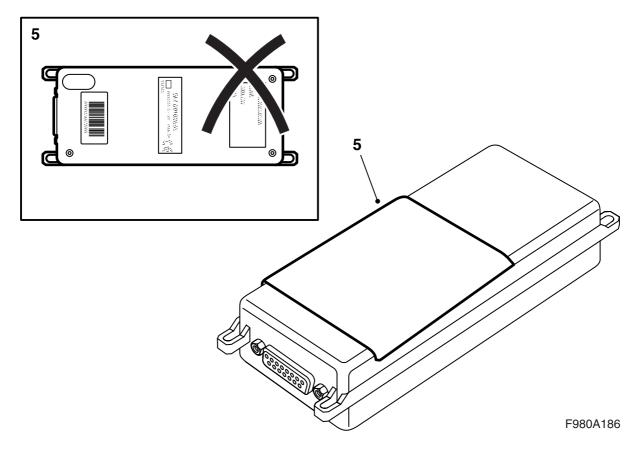
5 Cut one protective tape in the centre and fit one of the parts on top of the electronic unit.
