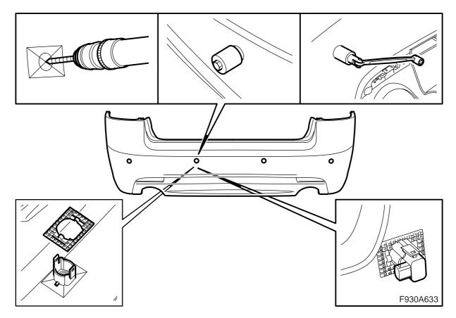
27 **M08**: Drill 8 mm holes (from the inside of the bumper shell) in the centre of each marking (x 4).
