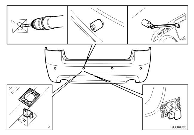
30 **M08**: Drill 8 mm holes (from the inside of the bumper shell) in the centre of each marking (x 4).
