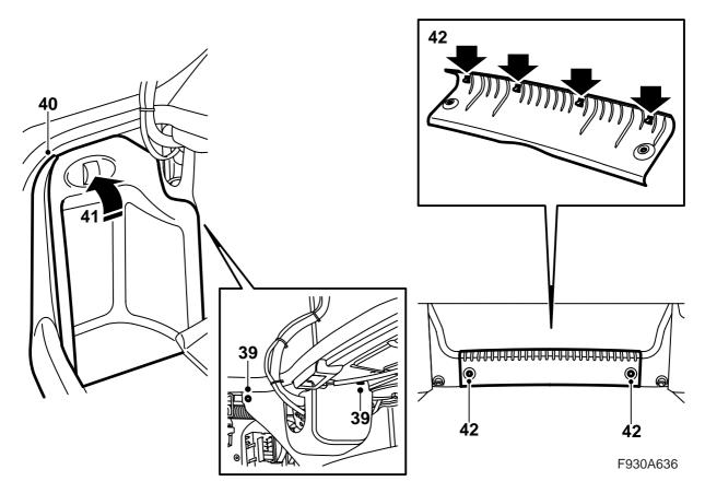
38 Fit the console in which such equipment as a CD changer/amplifier may be fitted. Plug in the connections to any equipment in the console.
