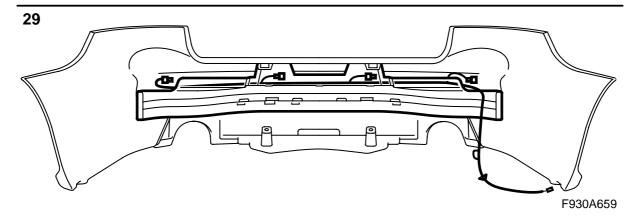
28 **M08:** Fit the wiring harness in the support for the bumper shell.
