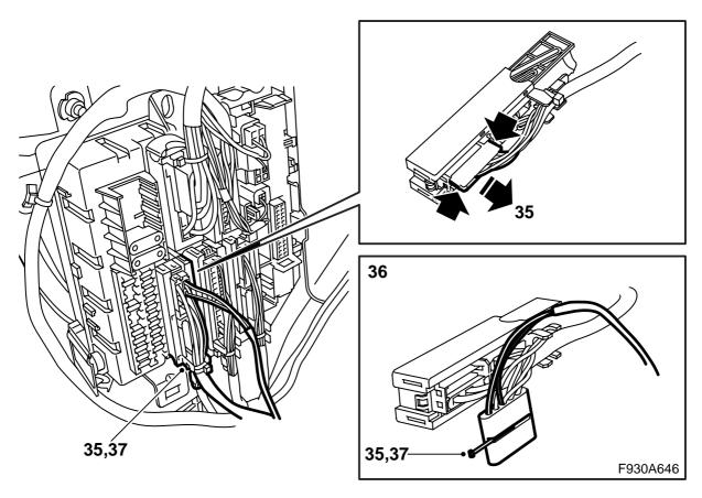
35 Remove the connector for the rear harness (blue) from the fuse box. Unplug connector A1 from the blue connector. Remove the lock.
