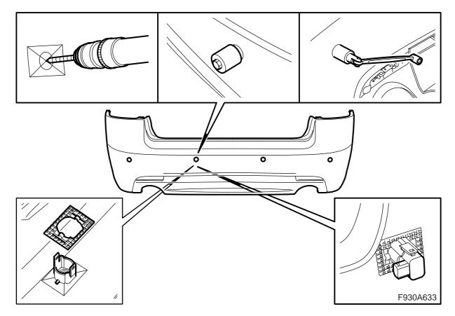
12 **M08:** Drill 8 mm holes (from the inside of the bumper shell) in the centre of each marking (x 4).
