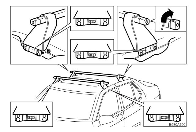
3 Start mounting on the left-hand side of the car. Carefully position the roof rack on the roof with the fixed supporting foot on your side of the car. Keep the supporting foot raised above the roof to avoid damaging the paintwork.
