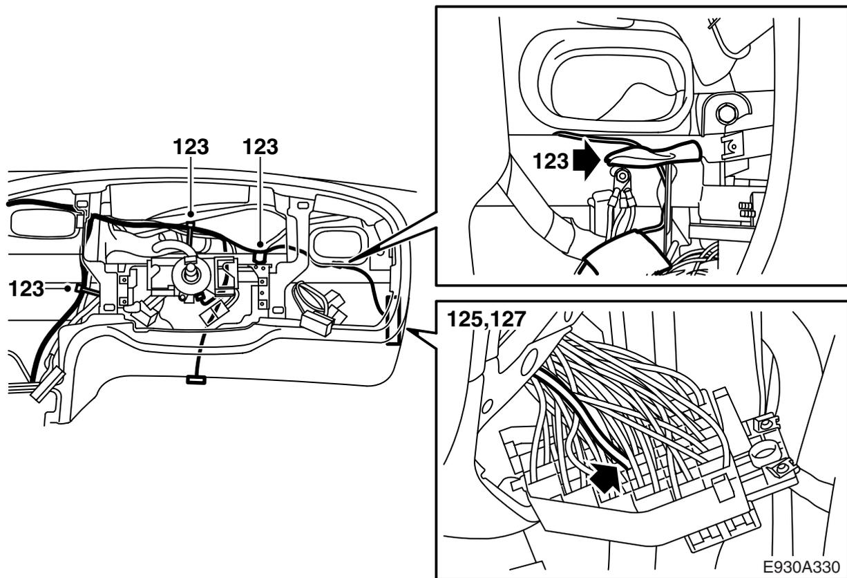
**123RHD:** Position the wiring harness branch, which runs to the data link connector, fuse box and driver's airbag connector, alongside the normal harness and secure with cable ties.
