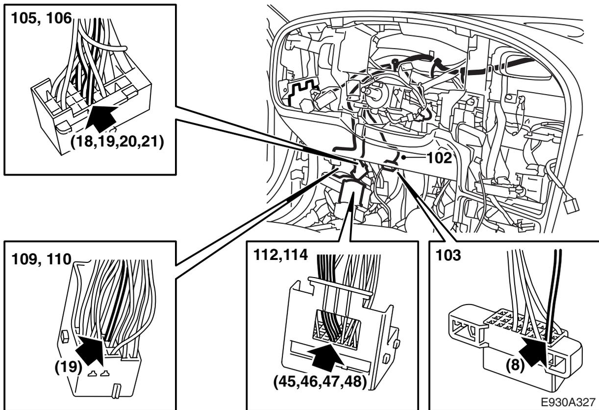
**102LHD:** Align the green wiring to the data link connector and secure.
