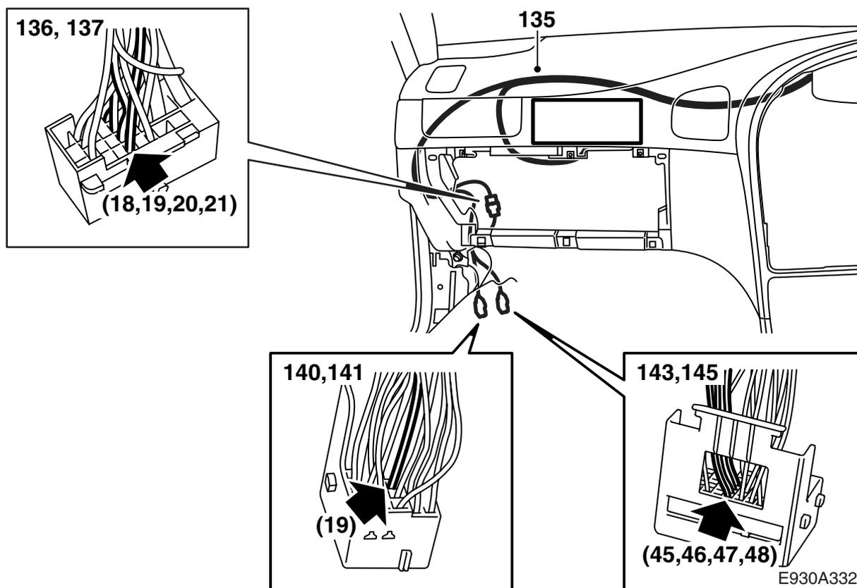
**135RHD:** Position the wiring harness down towards the connector bracket (166-pin connector), which is located down by the A-pillar. The harness must be routed behind the relay box. Secure and check that there is no risk of chafing.
