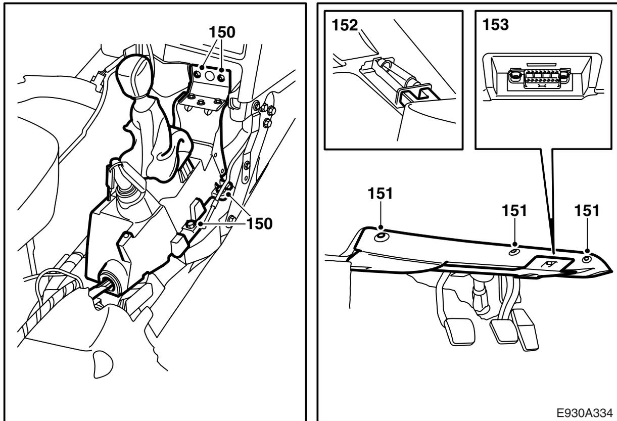
150 Fit the gear lever housing.
