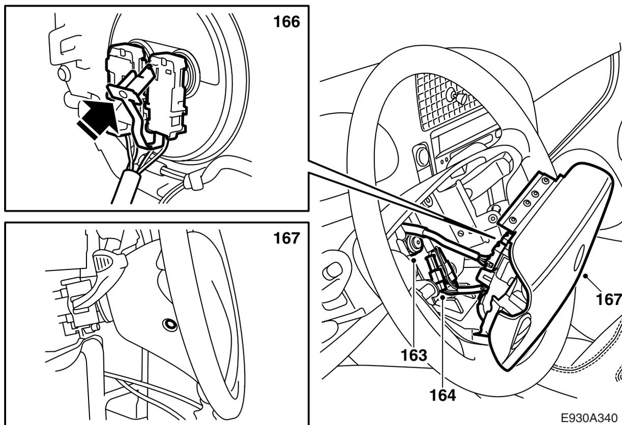
163 Fit and torque tighten the steering wheel nut.
