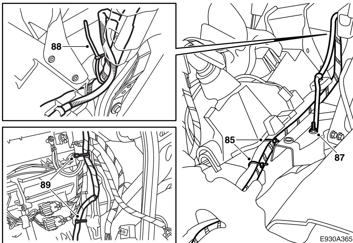
85 Secure the wiring harness with cable ties under the gear lever housing, along the normal harness. Check that there is no risk of chafing.
