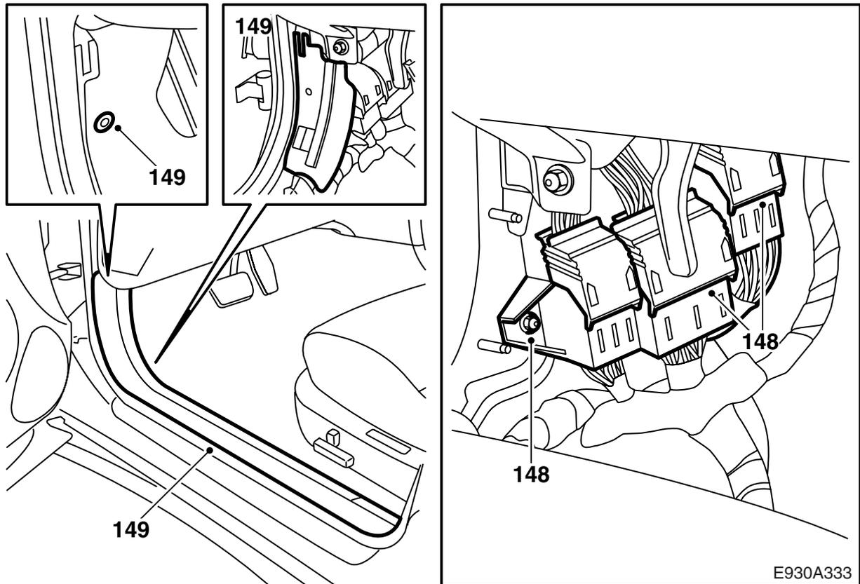
**148RHD:** Fit the connectors and screw back the bracket that holds the connectors.
