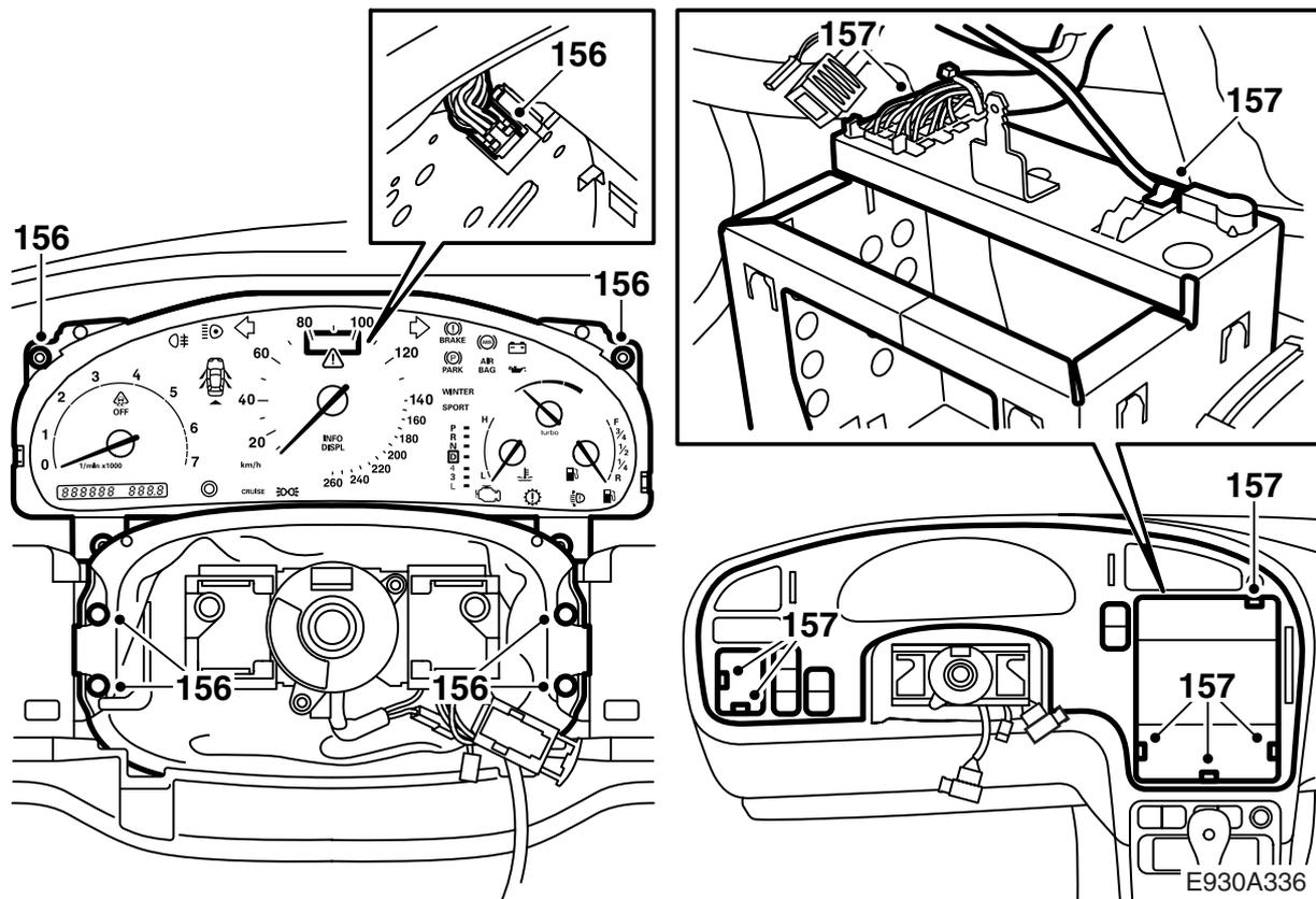
156 Fit the main instrument unit and the gaiter by the steering wheel.
