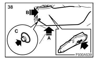
38 Fit the floor console's right-hand side piece.
