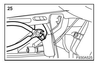
22.5 Fit the keypad and adjust any excess cable length.
