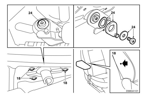
18 Fit the mounting into the seat.
