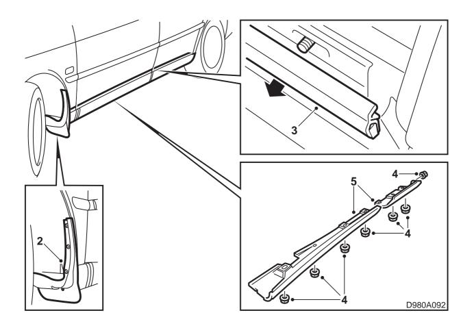
The installation instructions describe fitting on the left-hand side of the car. Repeat the procedure on the right-hand side.
