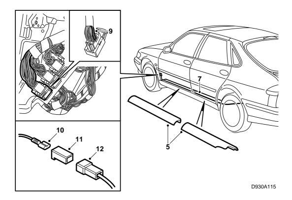
5 Remove the left-hand sill plates and cover under the steering wheel.
