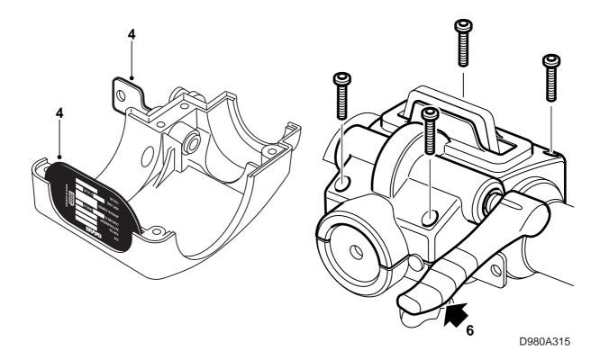
4 Insert a key in the lock and make sure it is unlocked, see the label. Place the type place in its recess.
