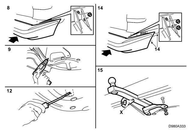
8 Mount the bumper, securing it with the two upper nuts.
