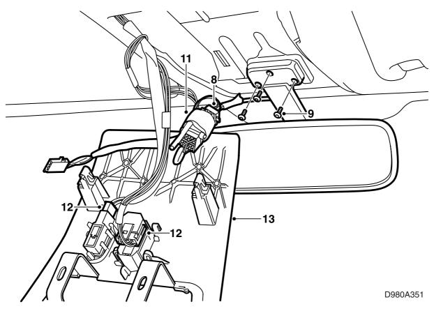
7 Carefully remove the tape from one connector on the kit's short wiring harness.
