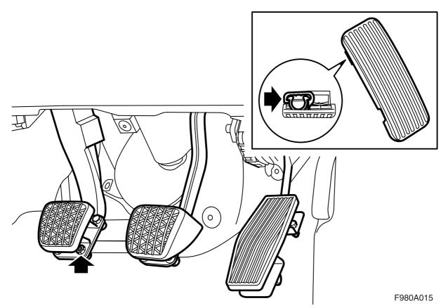
1 Remove the pedal pads from all the pedals **Accelerator pedal RHD:** Remove the entire pedal plate by releasing the clip and unhooking
