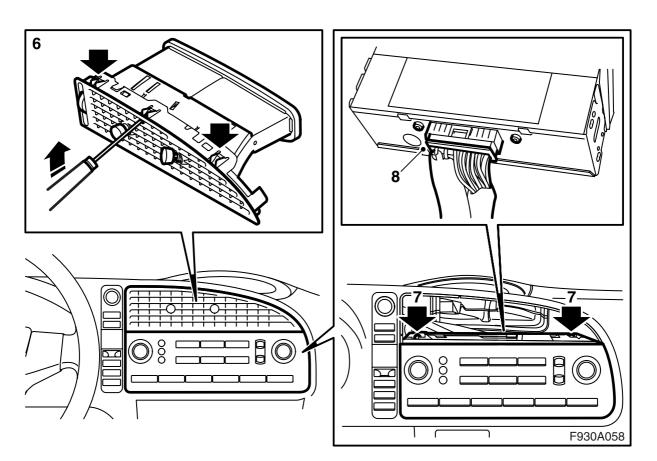
6 Remove the centre dashboard vent by carefully bending in the three upper hooks which are accessible through the grille while simultaneously pulling the guide pin straight out.
