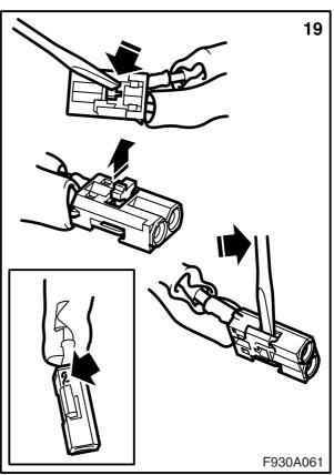
18 Remove the small connector from the large connector for the entertainment head unit.
