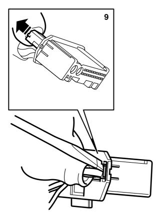
9 Remove the fibre optic cable connector (small connector) from the control panel connector.
