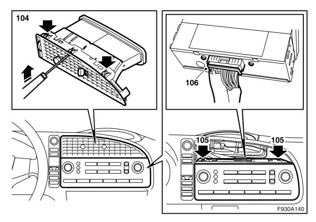
104Remove the centre air vent in the dashboard by carefully bending in the hooks accessible through the grille.
