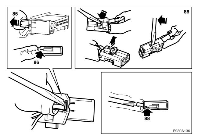
85 Bracket with amplifier or CD changer is fitted at the rear fuse box: Remove the amplifier or CD changer connector and remove the small connector from the large connector.
