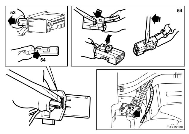
52 Cars where there is no bracket at the rear fuse box: Locate the green marked fibre optic cable at the amplifier.
