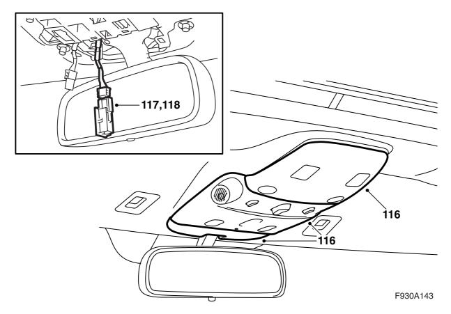
116 Cars without integrated telephone: Remove the rear, centre and front sections of the roof lighting cover. Tool 82 93 474 is recommended.
