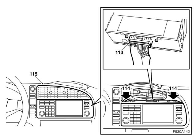
113 Connect the connector to the kit's control panel.
