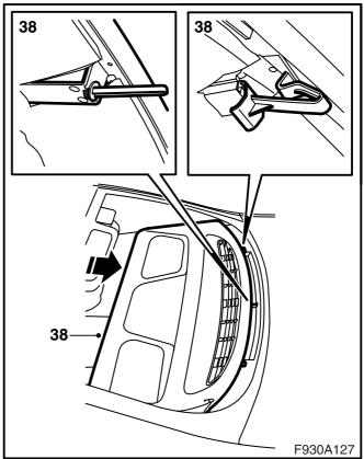
35 Position the C-pillar trim. Make sure that the screw with expander is in the correct position.
