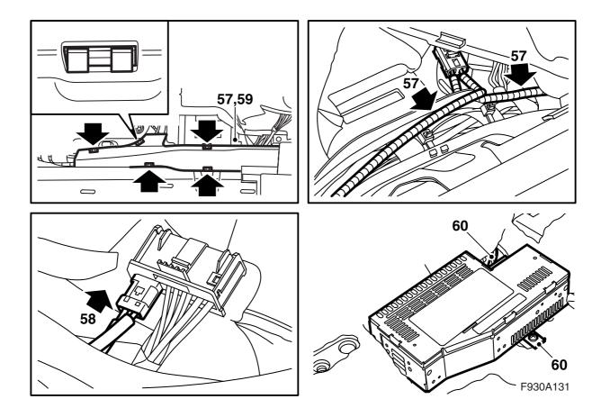
57 Cars where there is no bracket at the rear fuse box: Remove the cover on the cable duct, check that the fibre optic cable cannot bend and fit the connection on the fibre optic cable in position 1 in the small connector for the amplifier. Fit the lock.
