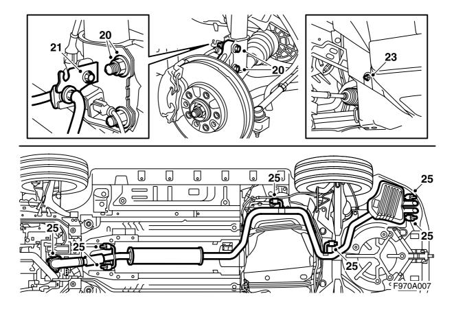
20 Raise the steering swivel member and push into place on the MacPherson strut. Fasten the steering swivel member to the MacPherson strut with new bolts, nuts and washers (the washers must be fitted on the same side as the nuts). Stop the bolt from turning with a spanner.
