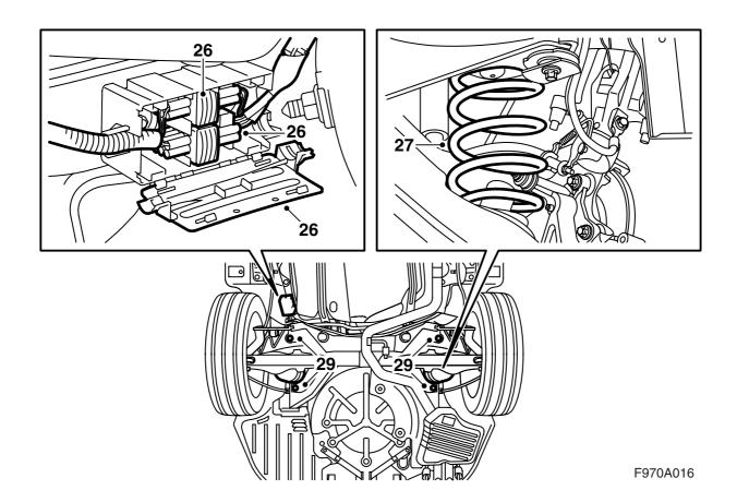
26 Plug in the wiring harness connector and close the lid of the protective box.
