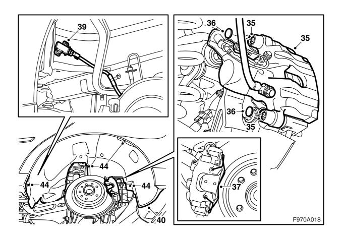
35 Fit the brake caliper.
