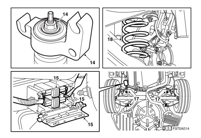
14 Fit the brackets to each of the shock absorbers with new nuts.
