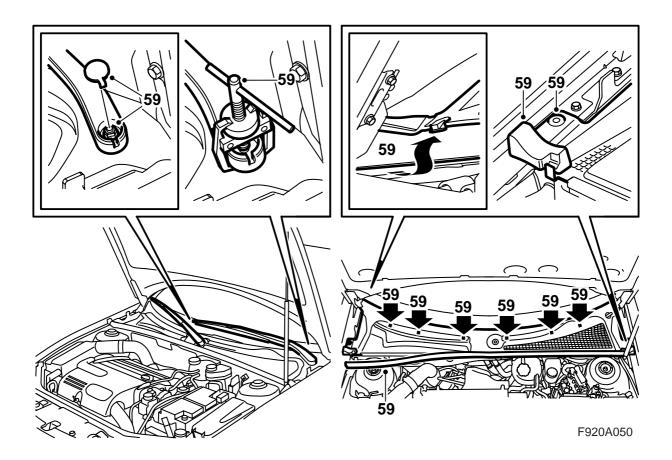
59 Remove the wiper arms using puller 85 80 144. Remove also the bonnet seal and the cover over the bulkhead space.
