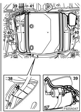
38 Remove the hose which is connected to the fuel filler pipe (the hose clip must be split with a saw) and fit the hose from the set.
