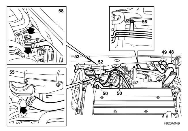
48 Fit the hose clips (including the old clip) onto the new coolant hoses. Connect the hose/pipe assembly between the thermostat housing connection and the heat exchanger connection nearest to the expansion tank. Do not screw the assembly to the bulkhead.
