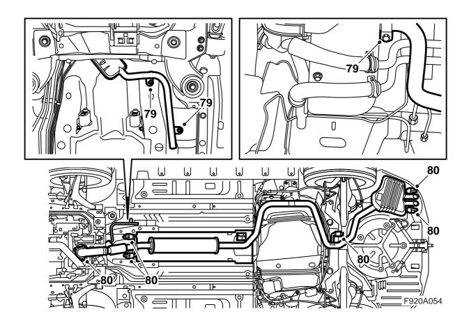
79 Manoeuvre the heater exhaust pipe up towards the heater and fit the end of the pipe onto the exhaust port of the heater. Fasten the exhaust pipe to the floor of the vehicle with the two nuts.
