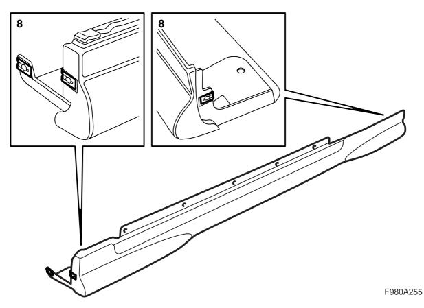
8 Fit the clip nuts in the front and rear edges of the sill covers.
