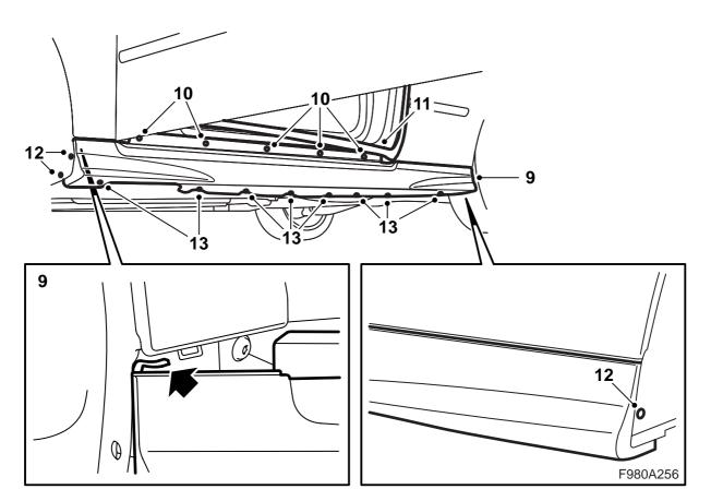
9 Pull out the front plastic wheel housing slightly at the rear edge, hook the sill cover securely into the front wing and press the sill cover securely at the back.
