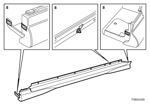
8 Remove the plastic clip from the old sill cover and fit it in the same position on the new one. Fit the clip nuts to the front and rear ends of the sill covers.
