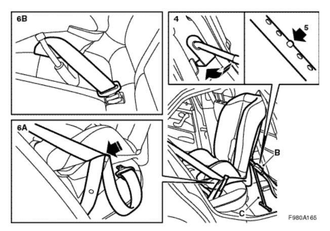
4 Fit the support (C) to the child seat by inserting the support's upper pipe end in the hole on the back of the child seat backrest and pressing the support down so that its snap locks catch in the child seat backrest.
