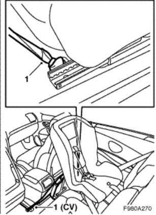
1 Secure the anchoring straps in the anchoring lugs at the car seat rails or around a member. See the Owner's Manual for the exact location. When fitting in the centre seat, the driver's/passenger seat attaching lug/member nearest the centre console should be used.
