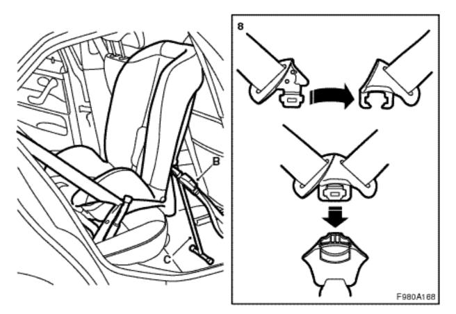
7 Secure the child seat with the anchoring straps (B) and pull them tight so that the child seat is stable. Make sure the support is steady against the floor of the car and the support lock button is in place in one of the holes.
