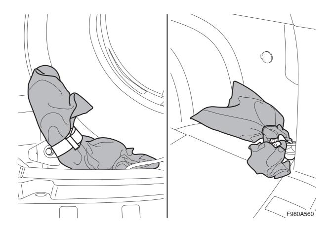
On the occasions when the ball unit is dismantled, it must be strapped into the eyelet in rear left-hand corner of the spare wheel well. If the car is equipped with large spare wheel then the ball unit must be strapped into one of the luggage compartment's load-securing eyelets.
