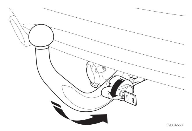
46 Fit the ball unit to the body bracket. Lock and remove the key.
