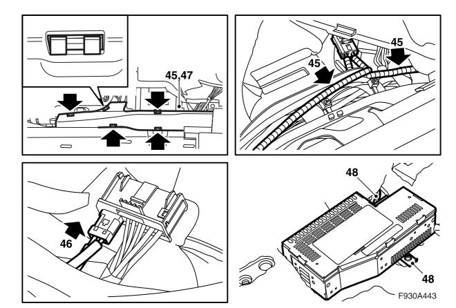
45 Remove the cover from the cable duct, check that the green marked fibre optic cable cannot bend and fit it in position 1 in the amplifier's fibre optic connector. Fit the locking clip.
