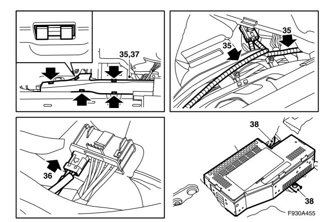
35 Remove the cover from the cable duct, check that the green marked fibre optic cable cannot bend and fit it in position 1 in the amplifier's fibre optic connector. Fit the locking clip.
