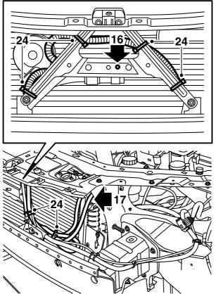
16 Drill a 6 mm hole in the horn bracket for the timer relay.
