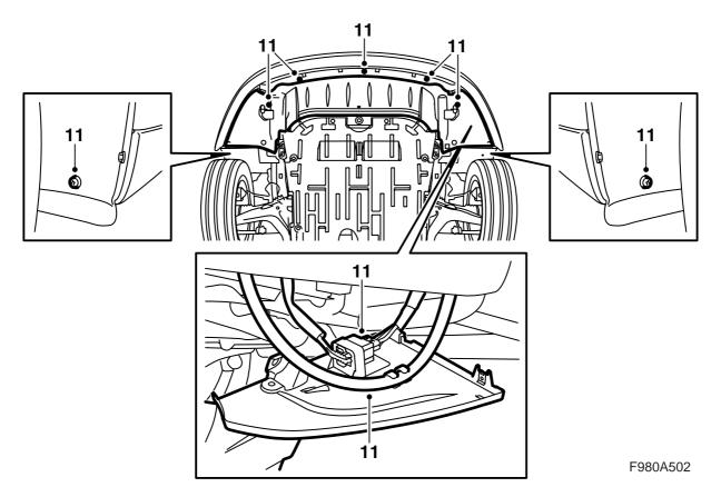
11 Fit the spoiler shield, secure the bumper connector and fit it to the holder on the spoiler shield.
