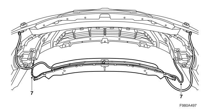
7 Secure the new wiring harness in the wiring harness duct and fit the clips.
