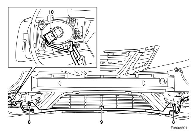
8 Fit the wiring harness duct.
