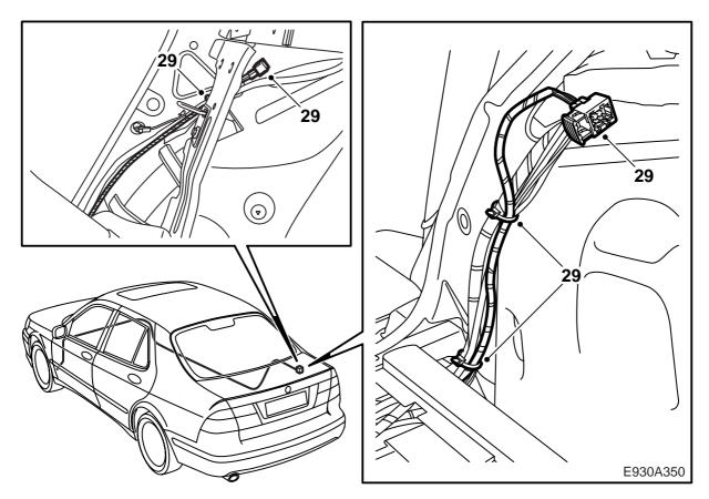
29 Route the kit's wiring harness beginning at the connector above the right-hand rear wheel housing, see illustration. Secure the connector with one cable tie at the connector housing and one at the sill duct.
