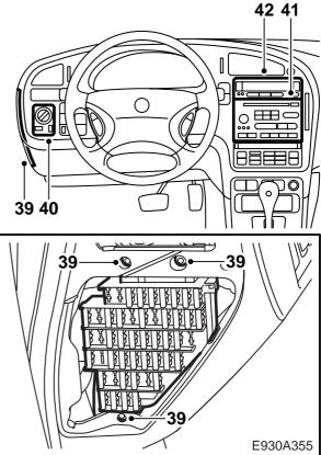
39 Fit the fuse box and the fuse hatch.
