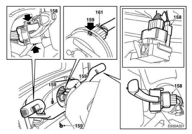
158Connect the connectors and fit the steering wheel switches.
