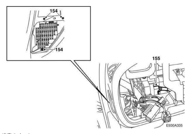
154Fit the fuse box.155Connect and fit the brown 33-pin connector.
