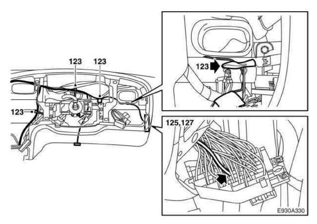
123RHD: Position the wiring harness branch, which runs to the data link connector, fuse box and driver's airbag connector, alongside the normal harness and secure with cable ties.
