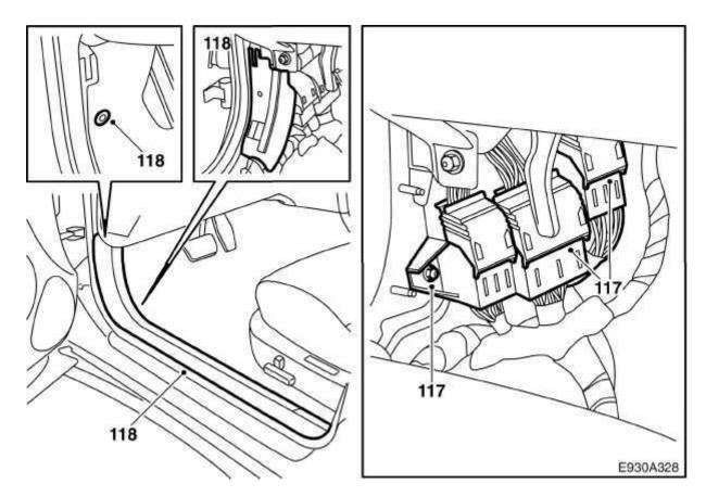
117LHD: Fit the connectors and screw back the bracket that holds the connector.
