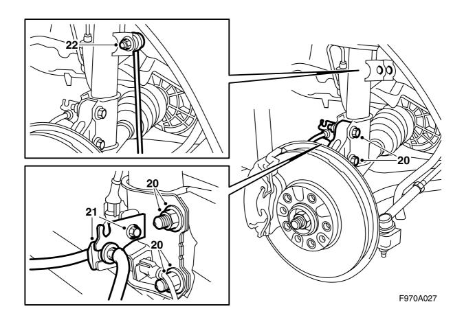
20 Raise the steering swivel member and push into place on the MacPherson strut. Fasten the steering swivel member to the MacPherson strut with new bolts, nuts and washers (the washers must be fitted on the same side as the nuts). Stop the bolt from turning with a spanner.
