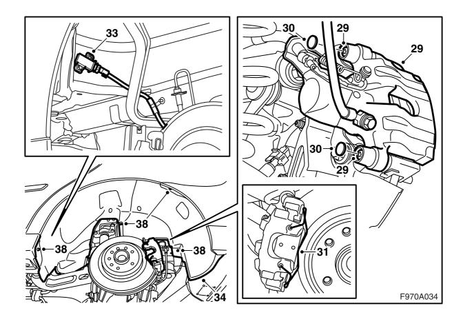
29 Fit the brake caliper.
