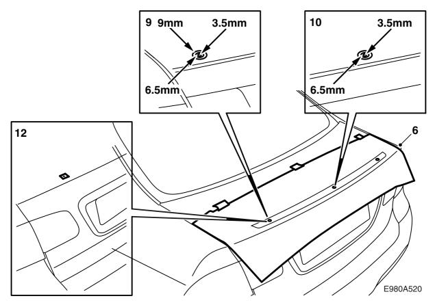
6 Cut out the template in accordance with the markings. Position the template on the boot lid and secure it with several pieces of tape.
