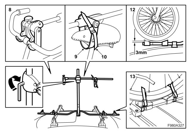
8 Secure the handlebars on the hooks, push the guide clamp down and tighten the clamp with the hand wheel.
