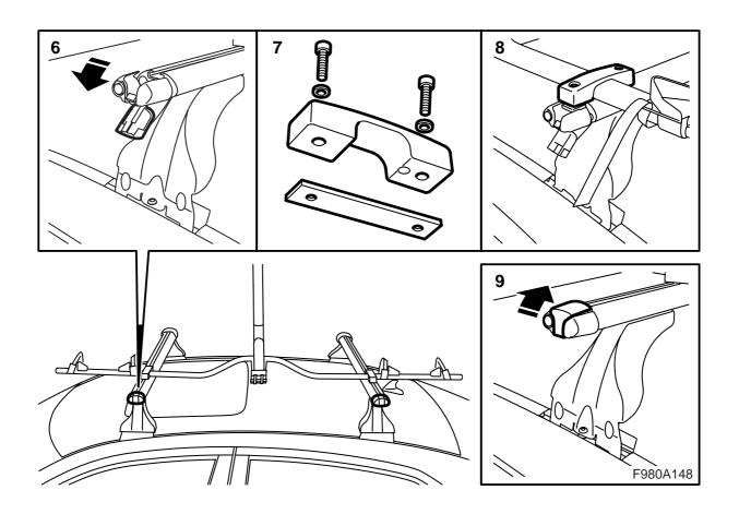
6 Pull out the carrier rack end plugs and fold down the centre section.
