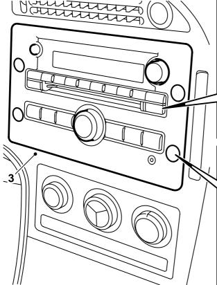
2 Plug the connector and antenna connection into the unit.
