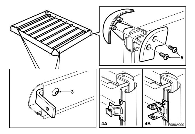
3 Fit together all frame sections with angle irons and screws. Begin by connecting the angle irons and the two loose frame sections (front and rear).
