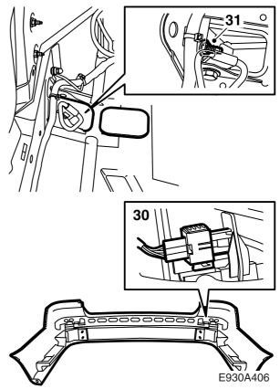
30 Fit in the bumper and plug in the connector.
