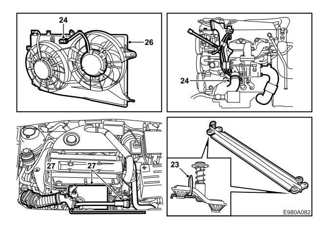
23 Press down the two spring-loaded holders for the radiator and charge air cooler and move them back towards the engine. Remove the holders.
