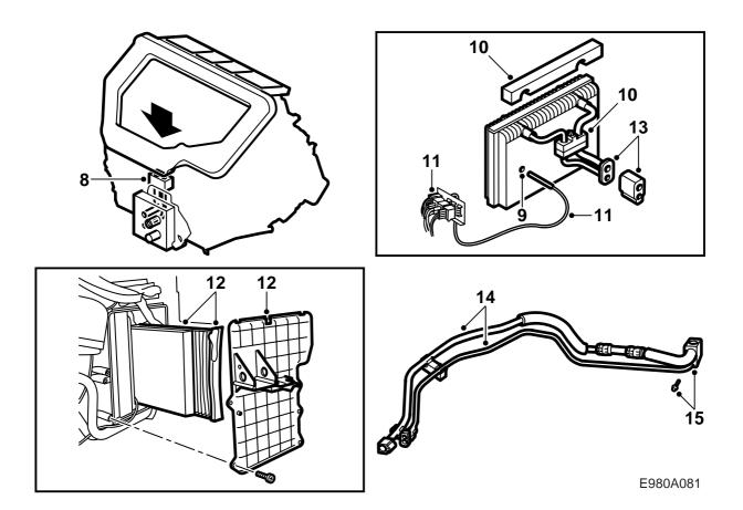
11 Remove the connector from the blind switch and pull off the rubber grommet from the sensor. Pull the sensor through the existing rubber grommet in the connector holder. Fit the connector into the connector holder and plug it into the existing wiring harness, 2-pin connector red/green and blue/white.
