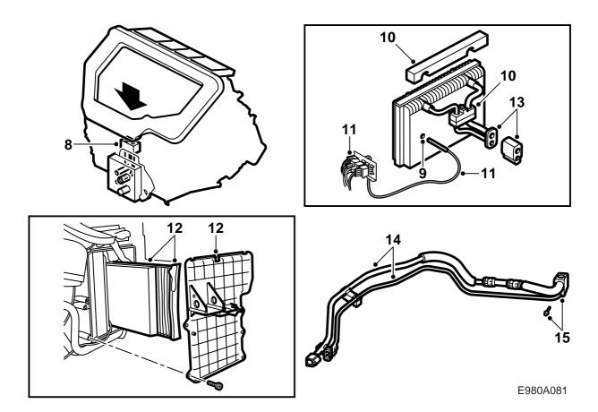
8 Pass the pipe from the evaporator housing through the bulkhead partition. Apply a little Vaseline on the pipes and push the pipe as far forward as possible to make room for the evaporator.
