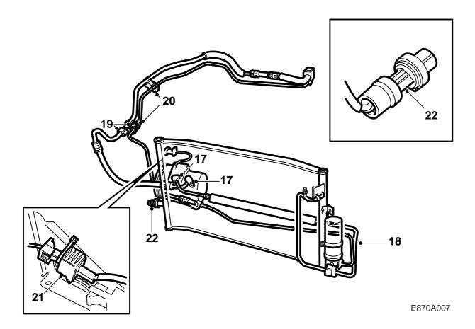
17 Remove the plugs from the compressor and the PAD attachments on the low-pressure and highpressure pipes. Lubricate the O-rings. Mount the low-pressure fitting on the compressor. Mount the high-pressure fitting on the compressor.
