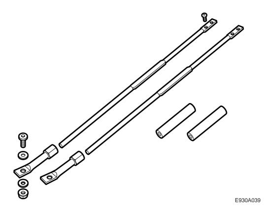
1 Stay including retaining screws and crimp hose
