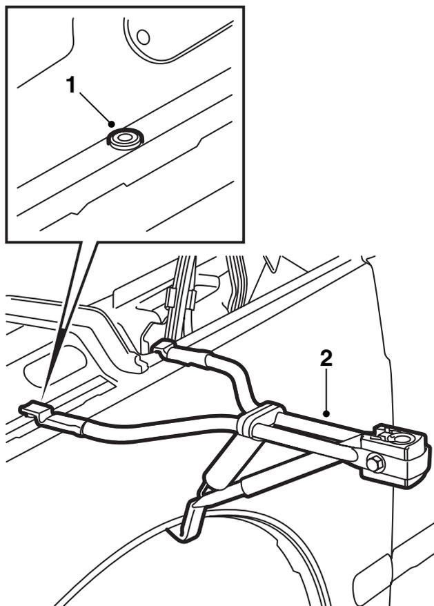
1 Open the bonnet and fit the rubber grommets into the holes, see illustration.
