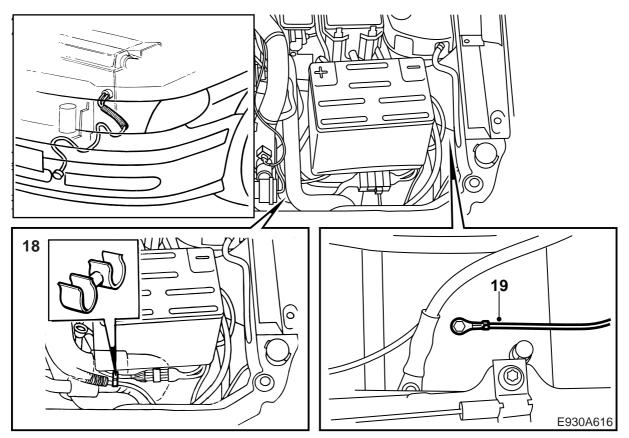
18 Secure the connector cable as illustrated.
