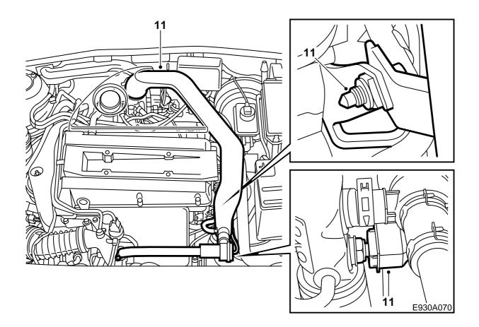
11 Remove the engine cover and disconnect any hoses and electrical connections from the turbo pressure pipe. Dismantle the turbo pressure pipe between the charge air cooler and the throttle body, including the by-pass pipe, as well as the heat shield above the exhaust manifold. Plug the holes.
