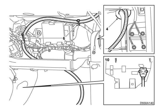
4 Pull the 2.0 m extension cable through the bulkhead.
