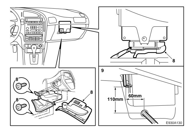
8 Remove the glove box and fold away the top of the carpet. If the glove box is cooled, detach the coolant hose.
