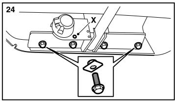
21 Remove the bolt fitted in one of the holes in the bumper rail and fit the towing bracket to the bumper. Check that the line above the upper bolts of the towing bracket is parallel to the bumper rail.
