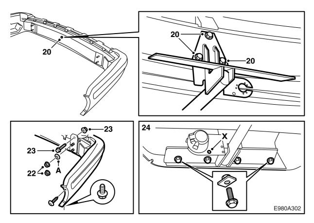
20 Remove the bolt fitted in one of the holes in the bumper rail and fit the towing bracket to the bumper. Check that the line above the upper bolts of the towing bracket is parallel to the bumper rail.
