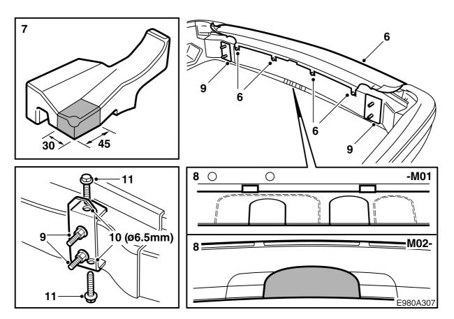
6 -M01: Slightly loosen the bolts of the upper portion of the bumper shell and carefully pull the upper portion of the shell out of its snap brackets.
