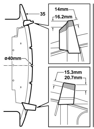
35 Cars with Vehicle Identification Number up to and including 33027678: Modify the spoiler shield.
