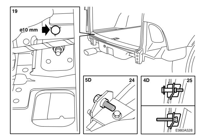
19 Use protective goggles and a 10 mm bit to drill through the sleeves, the holes in the rear end panel and the reinforcements.
