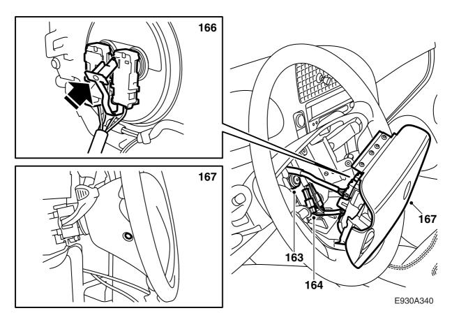
163Fit and torque tighten the steering wheel nut.
