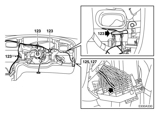
**RHD:** Position the wiring harness branch, which runs to the data link connector, fuse box and driver's airbag connector, alongside the normal harness and secure with cable ties.
