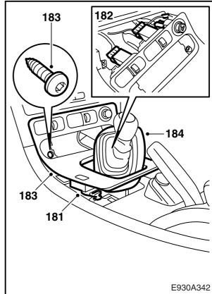
180Fit the electric window lift switches.
