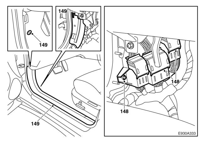
148**RHD:** Fit the connectors and screw back the bracket that holds the connectors.
