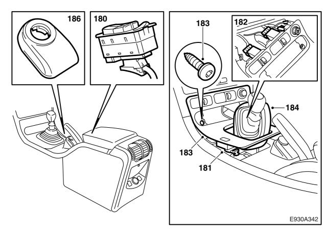
180Fit the electric window lift switches.
