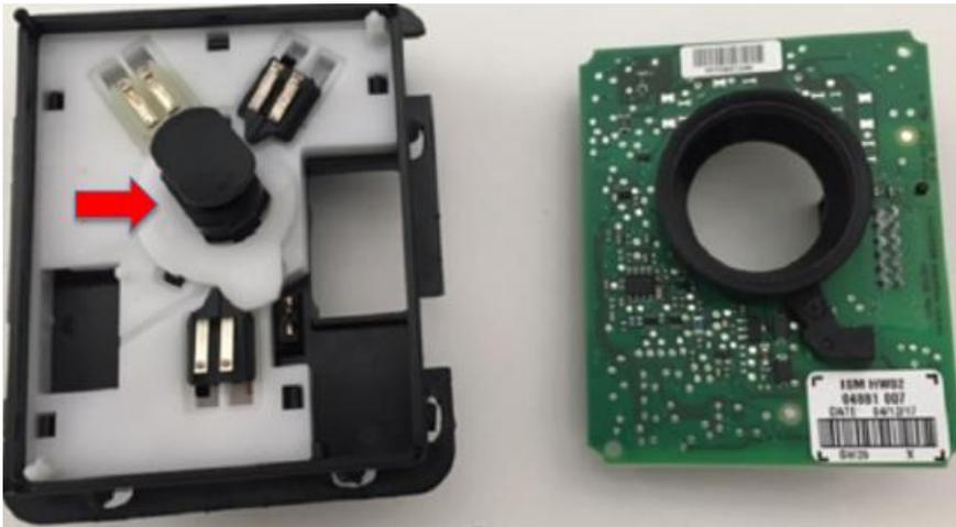
Install the circuit board with the connector side down. Make sure to align the pins to the holes in the circled areas.
