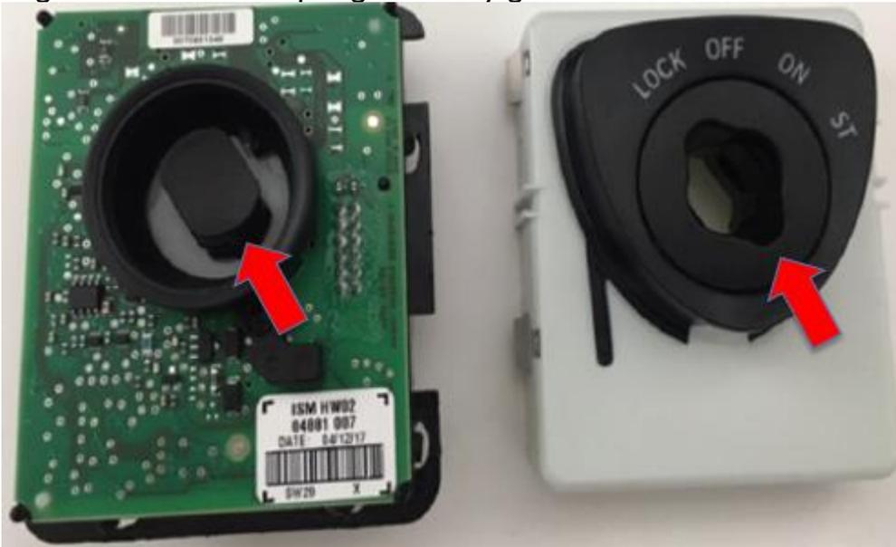
Once the alignment of the 2 housing is correct, slowly join them and snap together.
